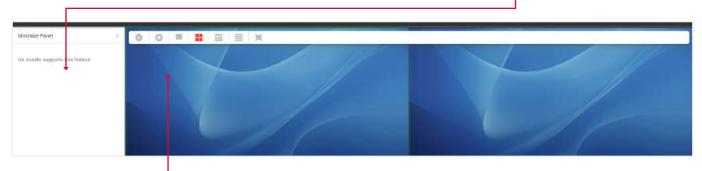
Above the camera display are buttons for turning **on** and **stopping** the video. Display **1,4,9** or **all** available cameras, as well as a **full-screen** video display option.
